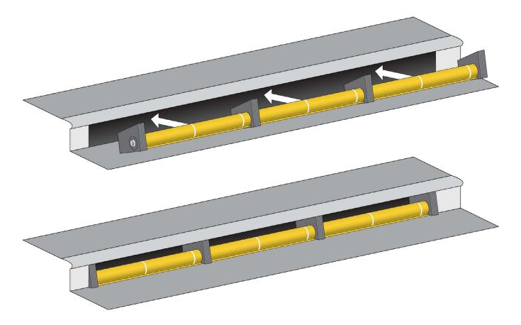
+ Note: The top of each Anchoring Wedge is perforated. If the Wedge is too large for the inlet, simply tear off the top section and reinstall (a second perforation is available if needed). The front of the Anchoring Wedges should be flush with the face of the inlet.
