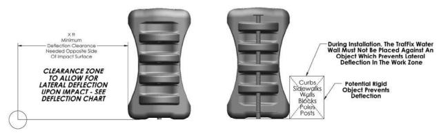
Figure 5: Clear Zone Diagram and Chart Recommendation
