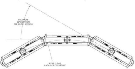
Figure 3: Angle of Rotation TrafFix Water-Walls Linked
