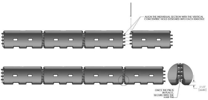
Figure 2: Installation Assembly Guide Diagram
