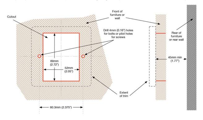
**Step 2.** Ensure HDMI and DC power are presented at the cutout and that you have sufficient slack to allow connection to the rear connectors on MediaHub UHD main unit. **Ensure the PSU is NOT plugged into the mains at this point.**
