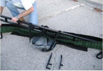
STEP 4: Slide assembled grids into outer sleeve.
