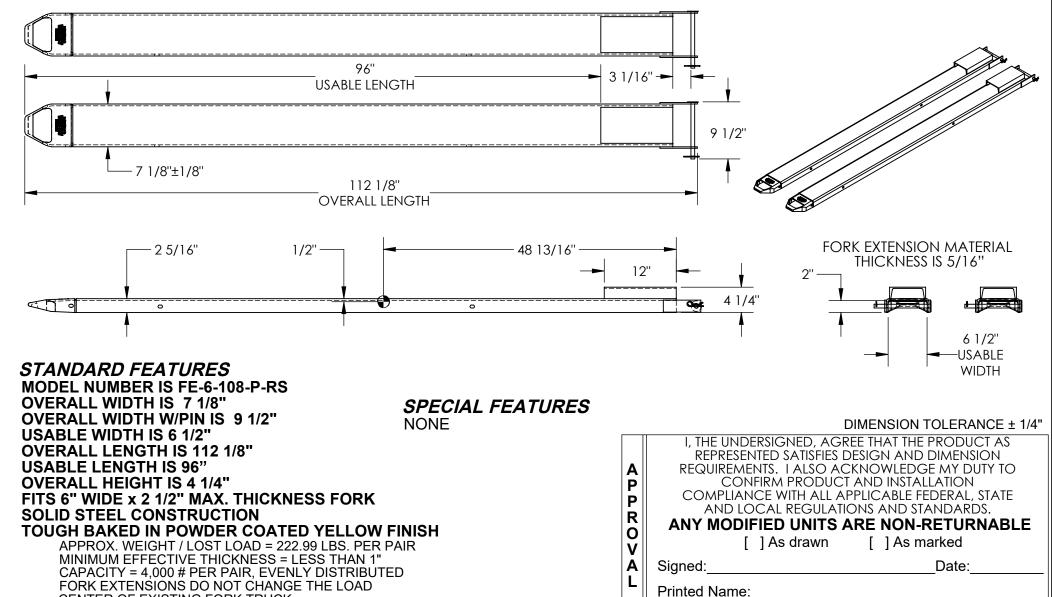
FORK EXTENSIONS DO NOT CHANGE THE LOAD CENTER OF EXISTING FORK TRUCK. NEVER EXCEED LOAD CENTER RATING PER FORK TRUCK MANUFACTURER'S GUIDELINES. DO NOT USE THESE FORK EXTENSIONS IF LOAD WILL EXCEED FORK TRUCK MANUFACTURER'S LOAD CENTER RATING. FORK EXTENSIONS MUST NOT EXCEED 150% ORIGINAL FORK LENGTH.
