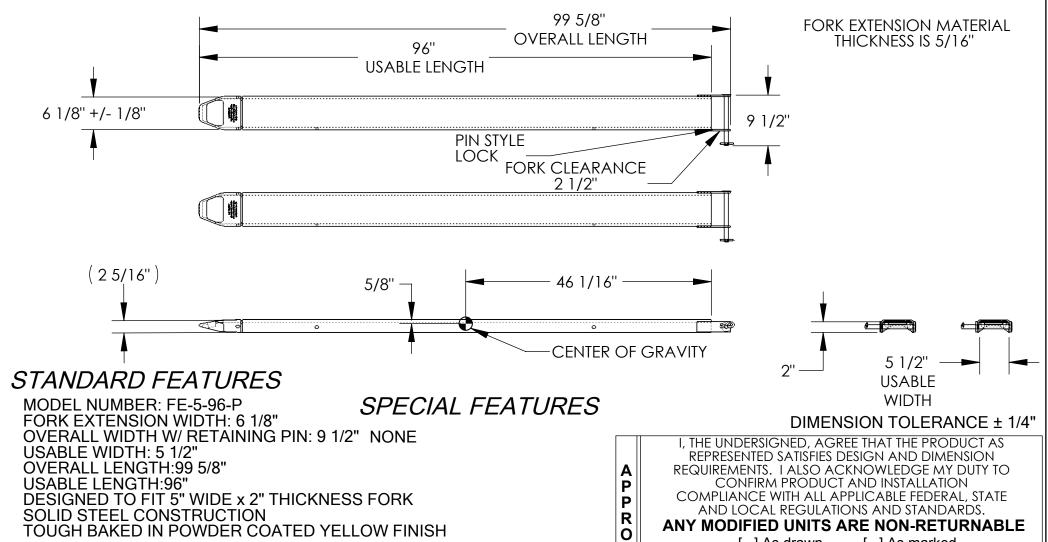
APPROX. WEIGHT / LOST LOAD = 167.28 LBS. PER PAIR MINIMUM EFFECTIVE THICKNESS = LESS THAN 1' CAPACITY = 4,000 # PER PAIR, EVENLY DISTRIBUTED FORK EXTENSIONS DO NOT CHANGE THE LOAD CENTER OF EXISTING FORK TRUCK. NEVER EXCEED LOAD CENTER RATING PER FORK TRUCK MANUFACTURER'S GUIDELINES. DO NOT USE THESE FORK EXTENSIONS IF LOAD WILL EXCEED FORK TRUCK MANUFACTURER'S LOAD CENTER RATING. FORK EXTENSIONS MUST NOT EXCEED 150% ORIGINAL FORK LENGTH
