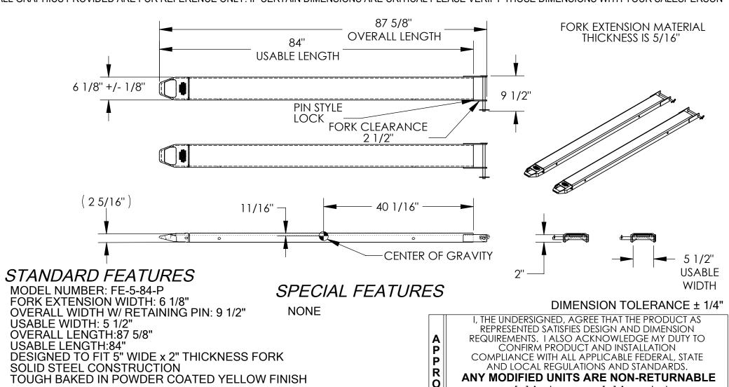
TOUGH BAKED IN POWDER COATED YELLOW FINISH APPROX. WEIGHT / LOST LOAD = 146.37 LBS. PER PAIR MINIMUM EFFECTIVE THICKNESS = LESS THAN 1' CAPACITY = 4,000 # PER PAIR, EVENLY DISTRIBUTED FORK EXTENSIONS DO NOT CHANGE THE LOAD CENTER OF EXISTING FORK TRUCK. NEVER EXCEED LOAD CENTER RATING PER FORK TRUCK MANUFACTURER'S GUIDELINES. DO NOT USE THESE FORK EXTENSIONS IF LOAD WILL EXCEED FORK TRUCK MANUFACTURER'S LOAD CENTER RATING. FORK EXTENSIONS MUST NOT EXCEED 150% ORIGINAL FORK LENGTH
