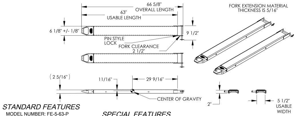
FORK EXTENSION WIDTH: 6 1/8" OVERALL WIDTH W/ RETAINING PIN: 9 1/2" NONE
