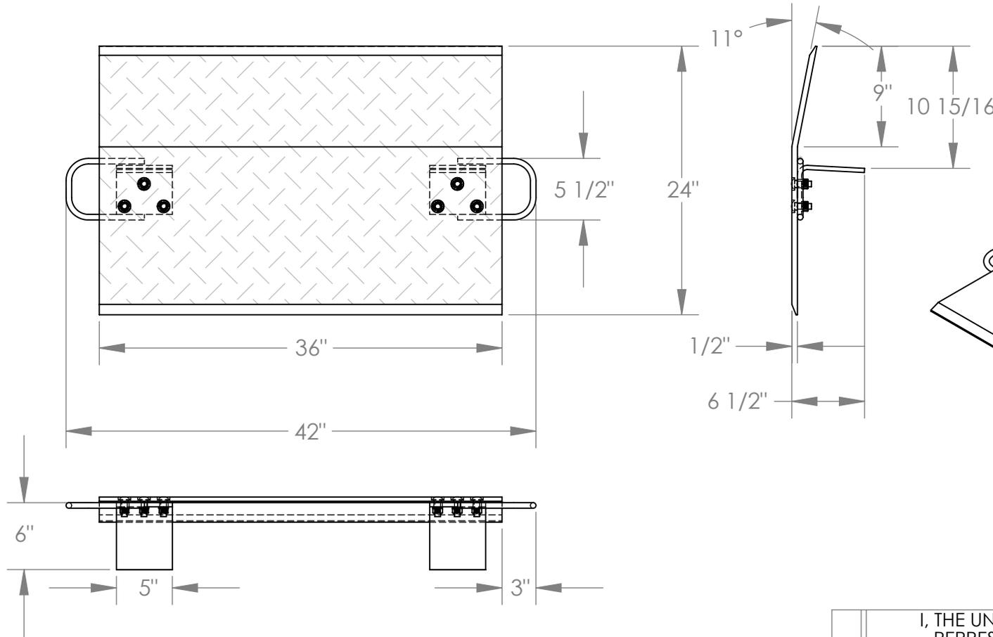
NOTE: BEND OR CROWN IS 11° AND LOCATED 9" FROM EDGE OF DOCKPLATE
