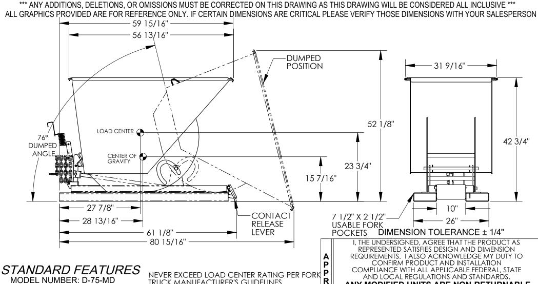
VOLUME: 3/4 CU. YDS. CAPACITY: 4,000 LBS. OVERALL WIDTH: 31 9/16" OVERALL LENGTH: 61 1/8" OVERALL HEIGHT: 42 3/4" PULL CABLE IS AT LEAST: 48" TOUGH BAKED IN POWDER COATED BLUE FINISH
