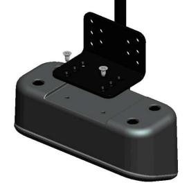
2. Position CubieMini on the back of the desk. Drill pilot holes at the desired screw location. A 1/16" or 3/32" drill bit should be used to reduce the risk of splitting the wood. Install wood screws (included) through bracket and into the pilot holes.
