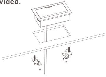
5. Secure CubieFlip<sup>™</sup> to the desk by tightening the 2 allen bolts.
